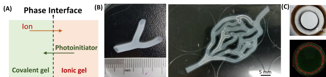
Figure 1. (A) Schematic of diffusion-induced gelation process for ionic and photo-crosslinkable hydrogels. (B) Representative tubular structure based on custom 3D printed mould. (C) Cross-section of multilayered heterogeneous tubular structures.
