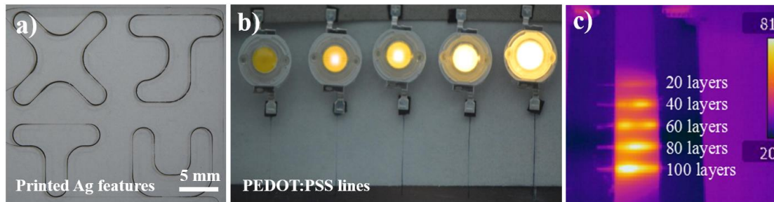
Figure 1. The EHD printed conductive features and the conductive/thermal property
