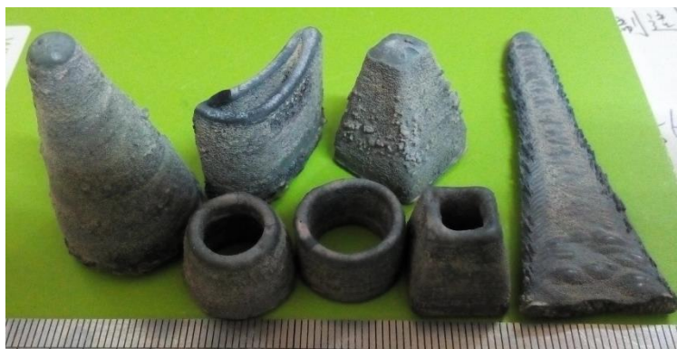
Figure 1. Alumina/aluminum titanate samples fabricated by DLD
