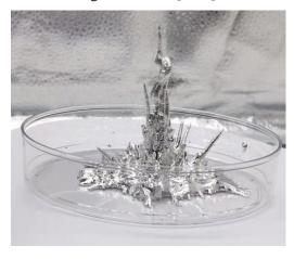
Fig. 1 Magnetic fluid based on liquid metal with the ability of solid-liquid transformation.
